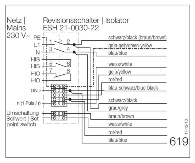
Wiring diagram for connection to: mains - service switch - motor
